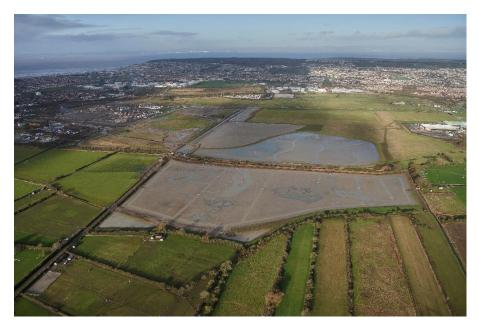
Reservoirs are where water is stored above normal ground levels. There is a slight risk that an embankment that holds the water above ground level could fail, and the water could escape and cause flooding. The management of reservoirs is heavily regulated to make sure the risk of any failure is minimal. Inspections are carried out by government appointed independent engineers.
